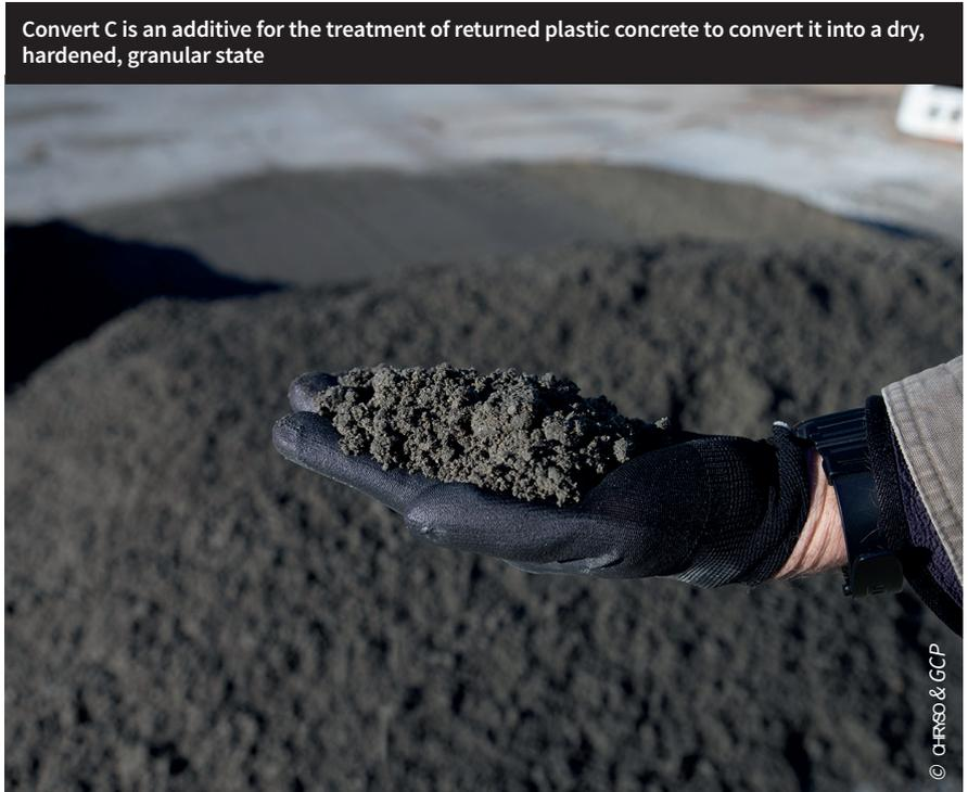
Convert C is an additive for the treatment of returned plastic concrete to convert it into a dry, hardened, granular state
